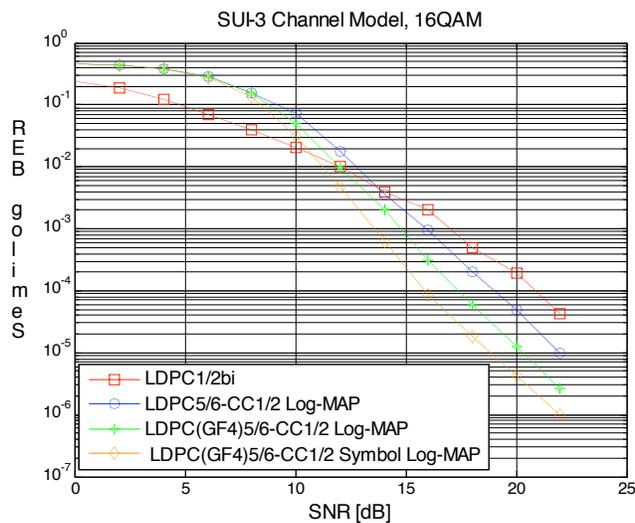
Fig. (11). Bit Error Rate of some LDPC and LDPC-CC concatenated codes over SUI-3 channel model.
