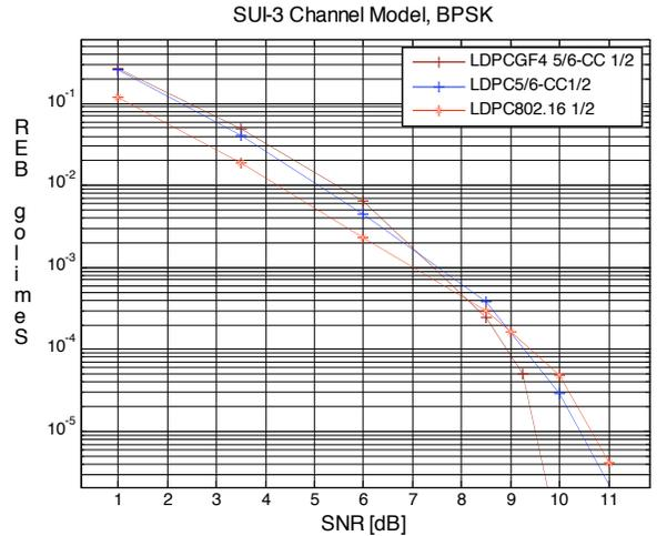
Fig. (9). Bit Error Rate of concatenated  $GF(4)$  LDPC-CC over SUI-3 channel model.
