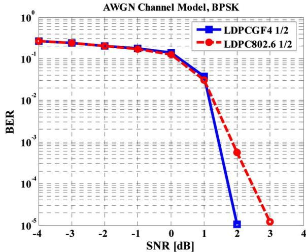
Fig. (3). Bit Error Rate for the rate  $\frac{1}{2}$  LDPC code of the IEEE 802.16 standard compared with the proposed  $GF(4)$  code over AWGN.
