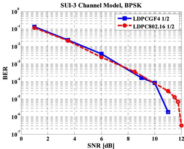
Fig. (4). Bit Error Rate for the rate  $\frac{1}{2}$  LDPC code of the IEEE 802.16 standard compared with the proposed  $GF(4)$  code over SUI-3 channel model.
