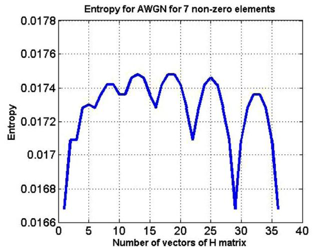
Fig. (2). Entropy over AWGN for 7 non-zero elements with probability of error  $10^{-5}$ .
