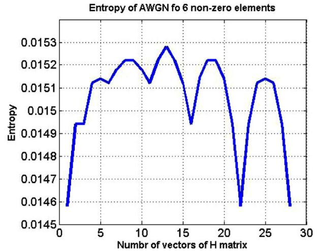
Fig. (1). Entropy over AWGN for 6 non-zero elements with probability of error  $10^{-5}$ .
