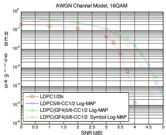
Fig. (10). Bit Error Rate of some LDPC and LDPC-CC concatenated codes over AWGN channel model.
