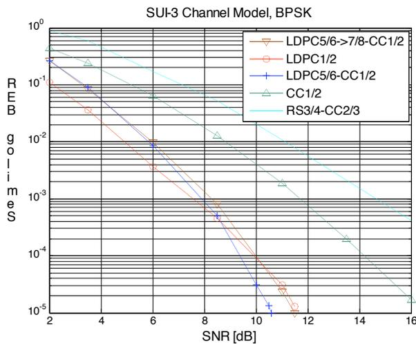
Fig. (8). Bit Error Rate of some LDPC-CC concatenated codes over SUI-3 channel model.
