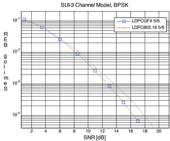
Fig. (6). Bit Error Rate for LDPC of IEEE 802.16 rate  $\frac{5}{6}$  using both binary and  $GF(4)$  with the proposed matrix over SUI-3 channel model.
